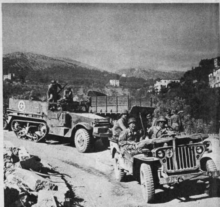
As a personnel carrier , this standard American M-3 half-track carries members of a rifle squad along an Italian road. The armored half-track may also be a prime mover of weapons up to 105-mm. in size.
